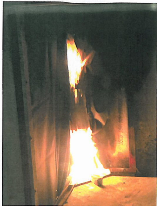
Figure 2 – The SBI test.
